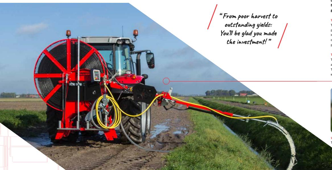
The DELTA offers more ease of use as a draincleaner than the JUNIOR. This is the ideal machine for anyone who maintains drainage systems on a frequent basis and needs to cover a large area. This is because it offers hydraulically operated height adjustment, extension, retraction and folding of the drainage arm and length adjustment of the guide arm.
